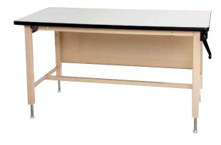
750 lb capacity vertical adjust station for applications that our standard 330 lb capacity Ergo Line does not address (Height range 11.812"). Standard height adjustment 30.375" to 42.187". Other heights available - Additional charges apply
