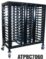
Adjustable Tray / PCB cart. Quickly reconfigure rack to transport different size trays or boards. Center uprights adjust left or right on .5" centers and lock with spring loaded pin. Horizontal rails adjust on 1.75" centers. Offset cam locks load into place for transport.
